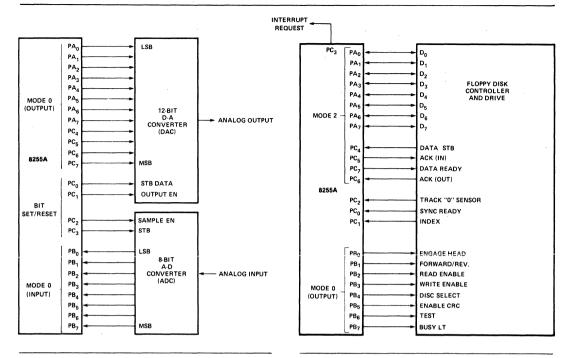
Figure 20. Digital to Analog, Analog to Digital
